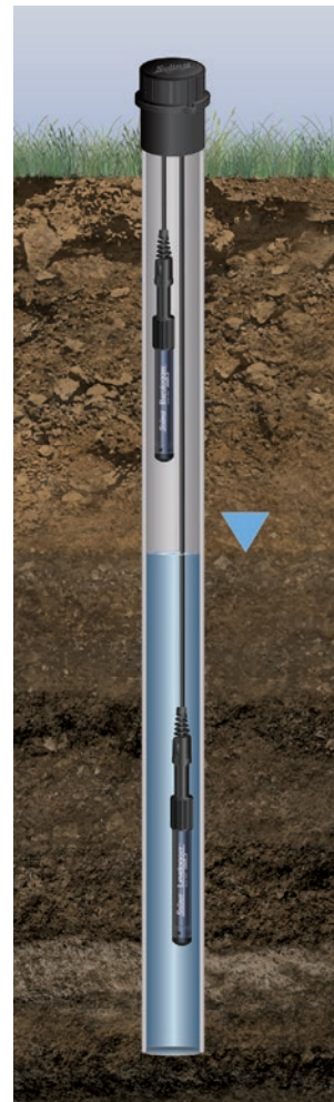
Barologger and Levellogger installed in Well Using Direct Read Cables
